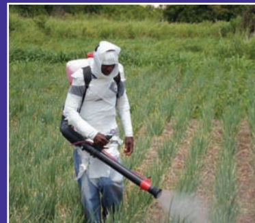
Figure 14. Pesticide applicator wrapped in paper to demonstrate drift of spray droplets during spraying of pesticide
